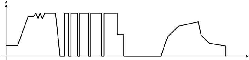
Additionally to the standard functions, which are all based upon a so-called arbitrary generator, this base generator is accessible for the creation and execution of complex sets of functions, separated into up to 99 sequences. These can be used for testing purposes in development and production. The sequences can be loaded from and saved to a standard USB flash drive via the USB port on the front panel, making it easy to change between different test sequences.
